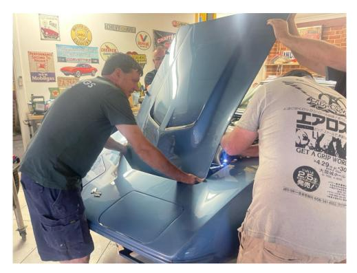
It was decided to remove the hood and remove the radiator and the associated brackets all in the one operation.
