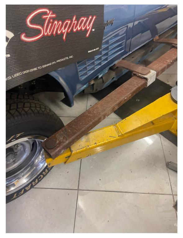
The system I use with my 2-post hoist, is I made up this 150 x 50mm RHS and located 50mm steel pins through it, into the holes on the hoist frame to support the RHS. I then made sliders that can be poisoned anywhere on the RHS with a 12mm x 200mm Welded to them, I then have a 90 deg, by 60mm turnup. This then can make contact with the bottom of the birdcage, so we are lifting the whole car by the bird-cage.
