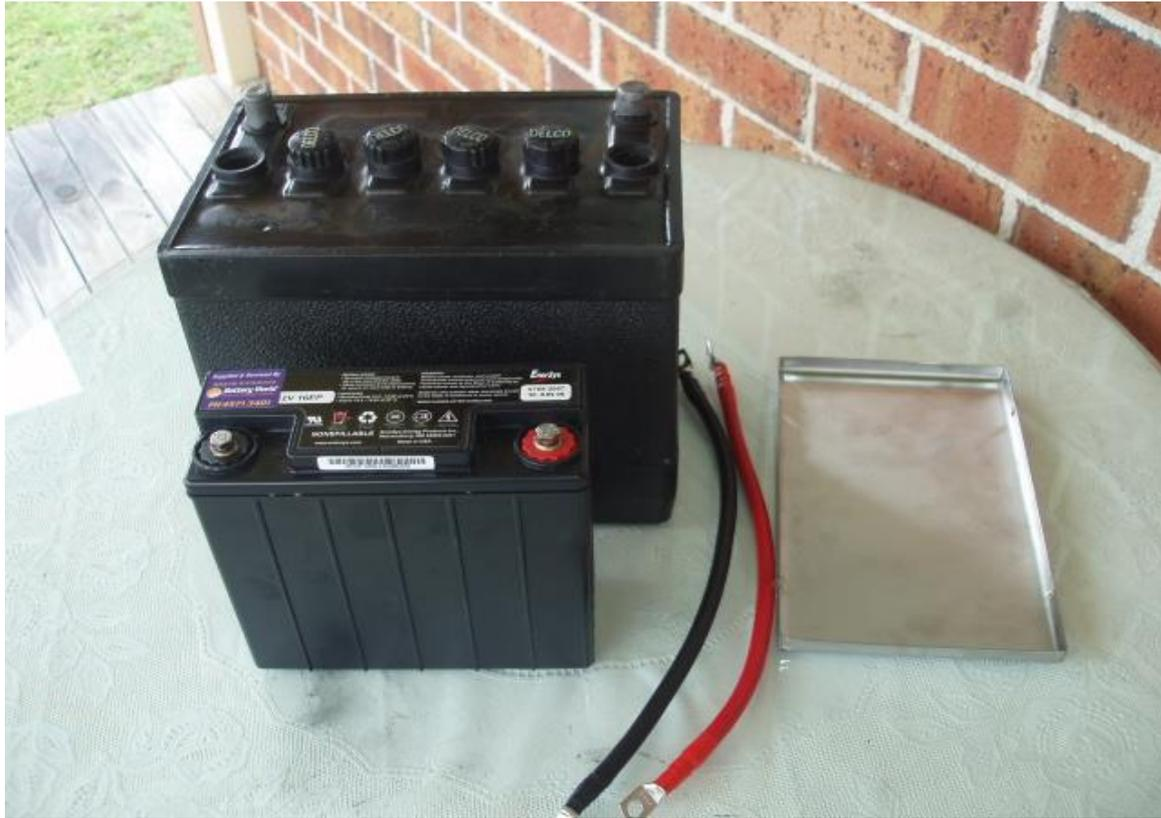
It was now time to connect the two terminals together. What I used here was two battery cables with lugs on both ends. Because I needed to bolt one end to the terminal inside the old battery and then bolt to the corresponding terminal on the new battery, it is better to bolt lugged cables to the original terminals rather than soldering them on as the solder may break off with vibration, as shown in the next photo;
