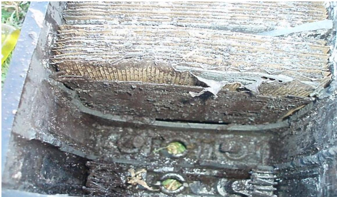
With a sharp wood chisel I was able to remove the two side dividers, exposing the next set of plates. Now I have more room I can remove the plates one by one till I have that section is cleared.
