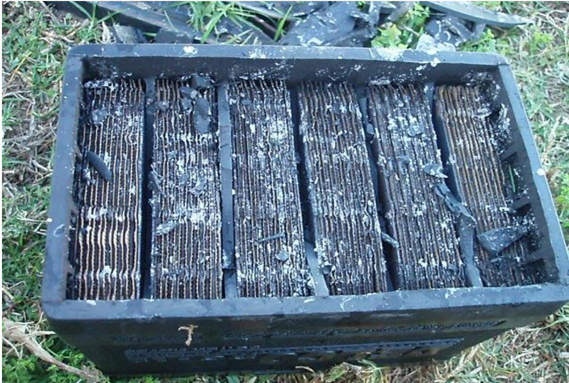
This process did take a long time, because it was very hard to remove as the plates would break up easily. After a while I was able to have a clear cavity in the battery. As shown in the next photo;
