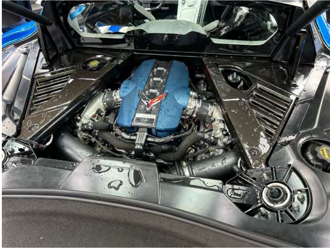
Here is a photo of the motor which is rated at 1064 HP.
