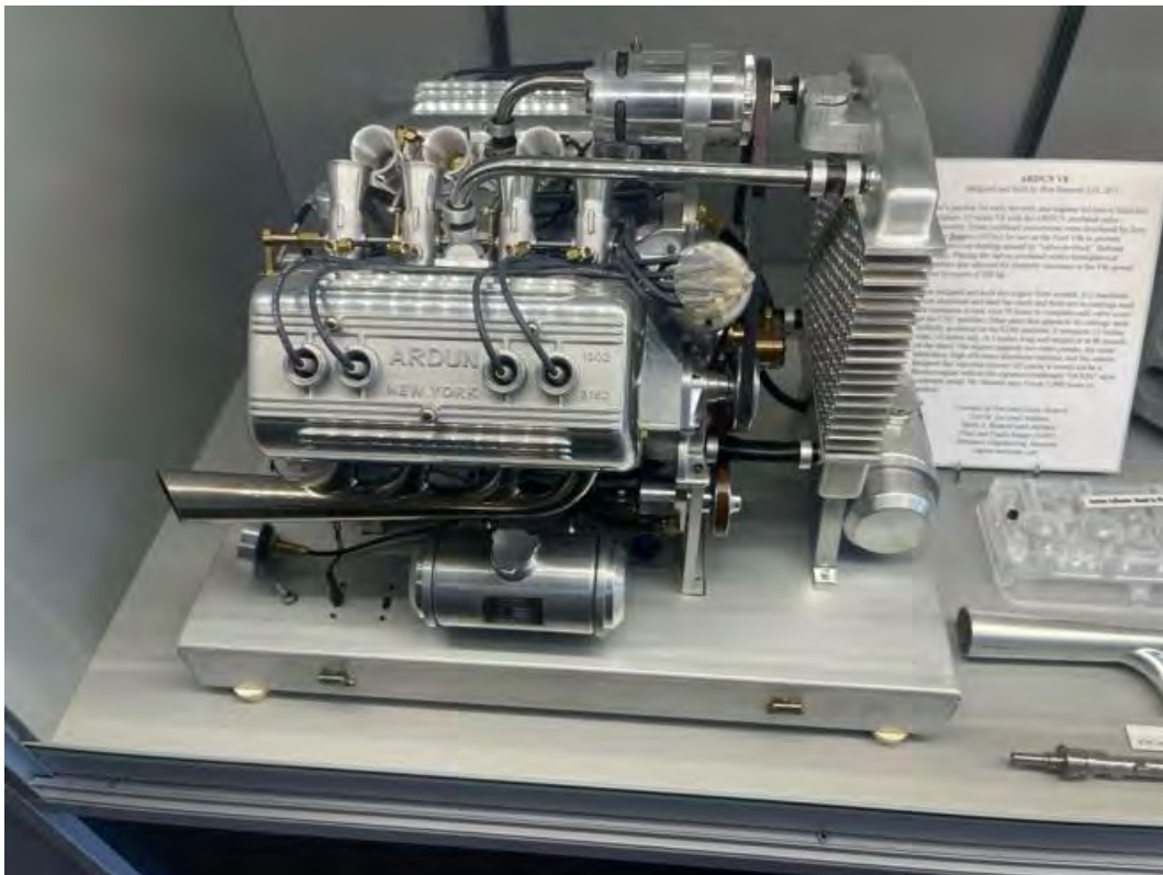
This engine has a set of Ardun heads on it.
